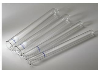
To suit different applications and manual/automatic handling systems, tubes for the digestion units are available in three sizes (400 ml, 250 ml and 100 ml) and three shapes. Straight sided tubes are recommended for the majority of digestion applications. Volumetric tubes with a constriction at the neck are recommended for applications where the digestate requires dilution to a fixed volume before analyses such as FIA, SFA, and AA etc.
