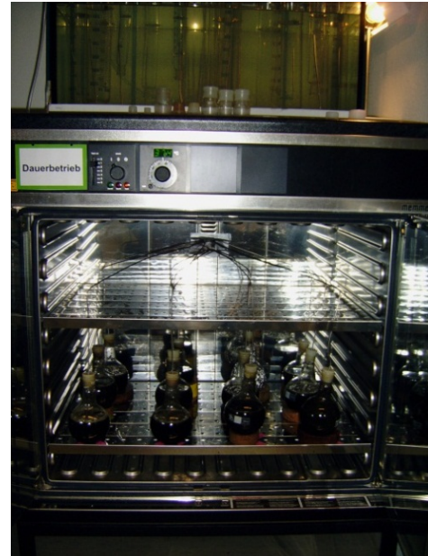
Fig. Experimental setup to generate bio gas in the laboratory
