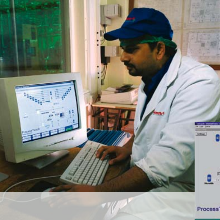
The heart of the FOSS Standardising solution – the ProcessTouch™ – links the PSC and the PLC together
